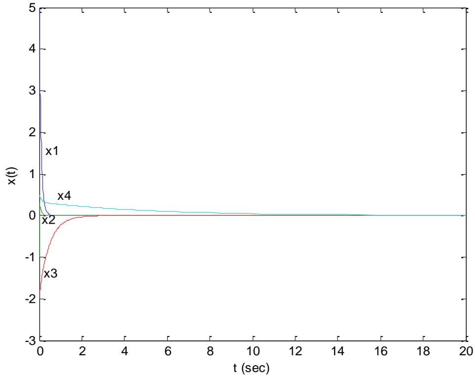
Figure 6: Typical state trajectories of the feedback-controlled system of Example 2.
