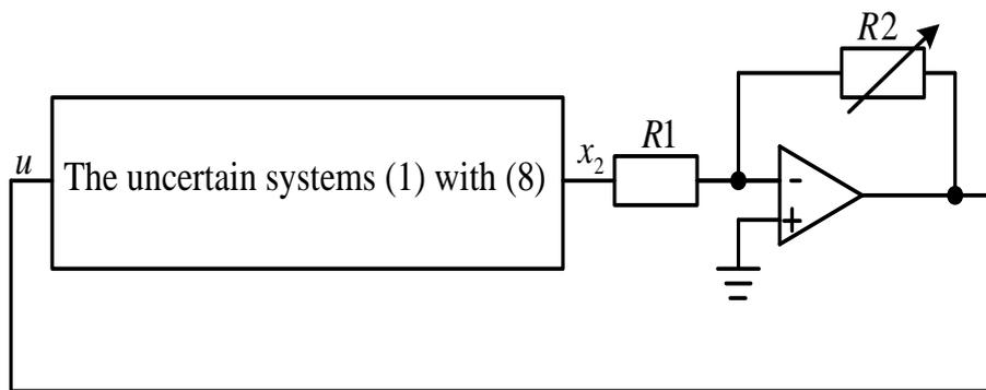
Figure 8: The diagram of implementation of Example 2, where  $R1 = 1k\Omega$ ,  $R2 = 351k\Omega$ .
