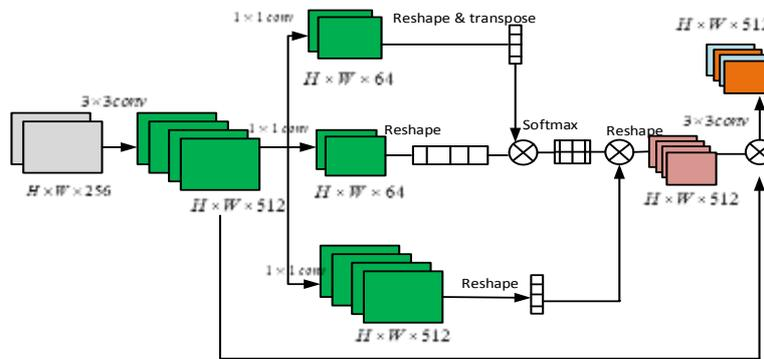
**Figure 3: Block diagram of position-wise attention block**
