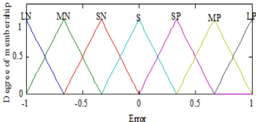
Fig 10 Membership function used for input variable “error”
