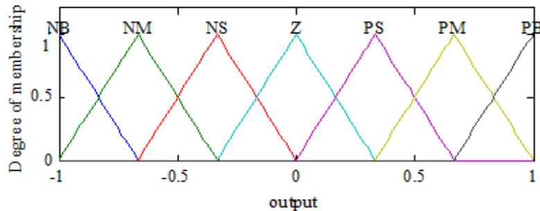
**Fig 12 Membership function used for output variable “output”**
