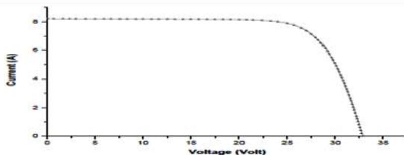
Figure 3 Characteristics of a PV cell
