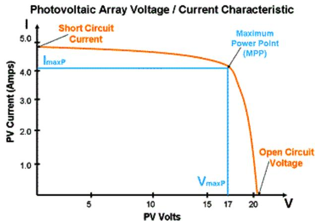
Figure 5 PV Characteristics With MPPT
