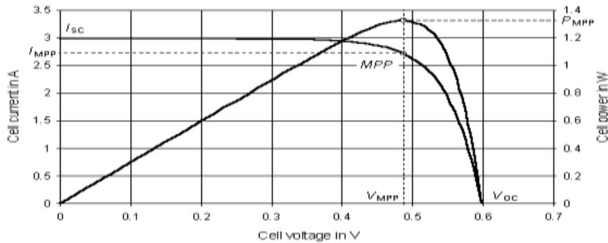
Figure 4 PV characteristics of Solar Cell
