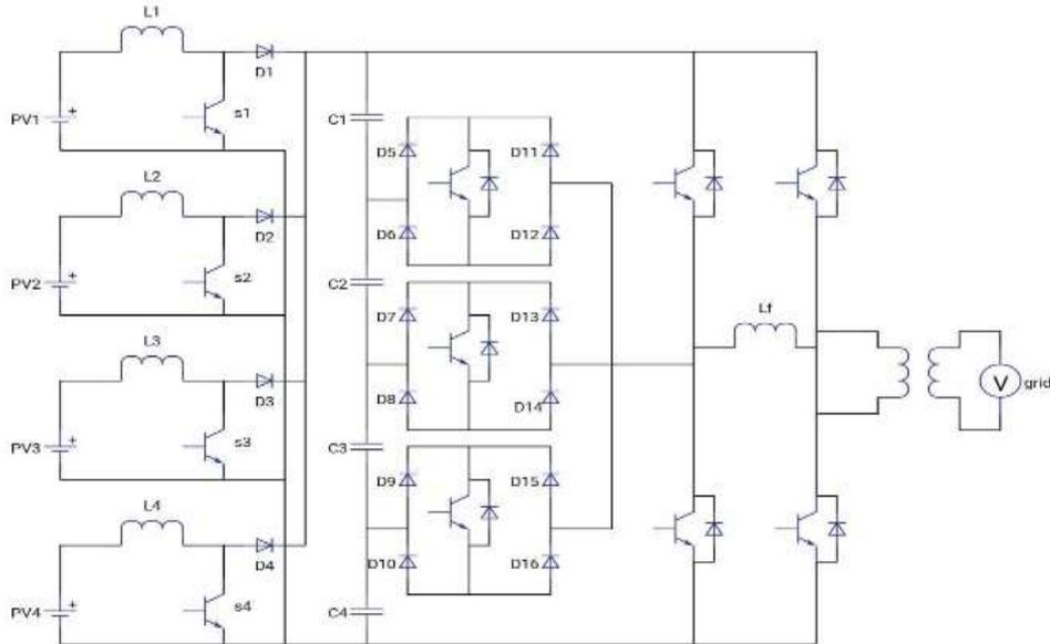
Fig. 2 proposed Multi-String Nine Level schematic diagram
