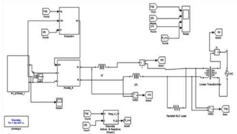
**Fig. 13 Simulation Diagram of Modified Nine Level inverter with PV String Module**
