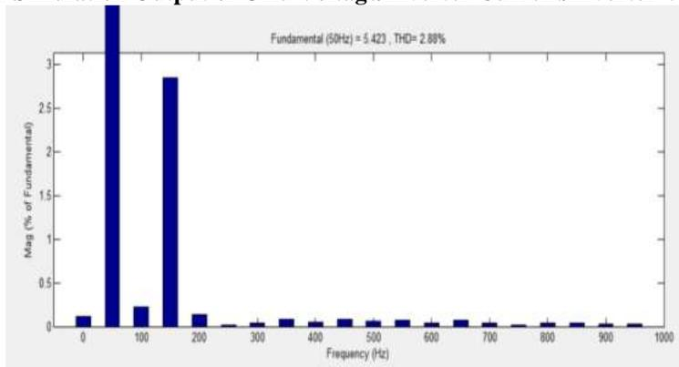
**Fig.23 Simulation Output of Proposed MLI THD Value after compensation period(2.83%)**
