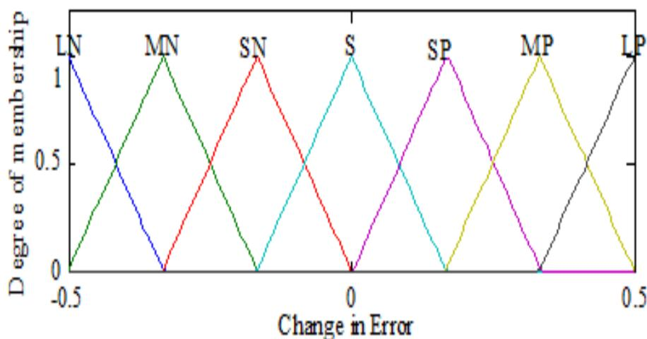
Fig 11 Membership function used for input variable “change in error”
