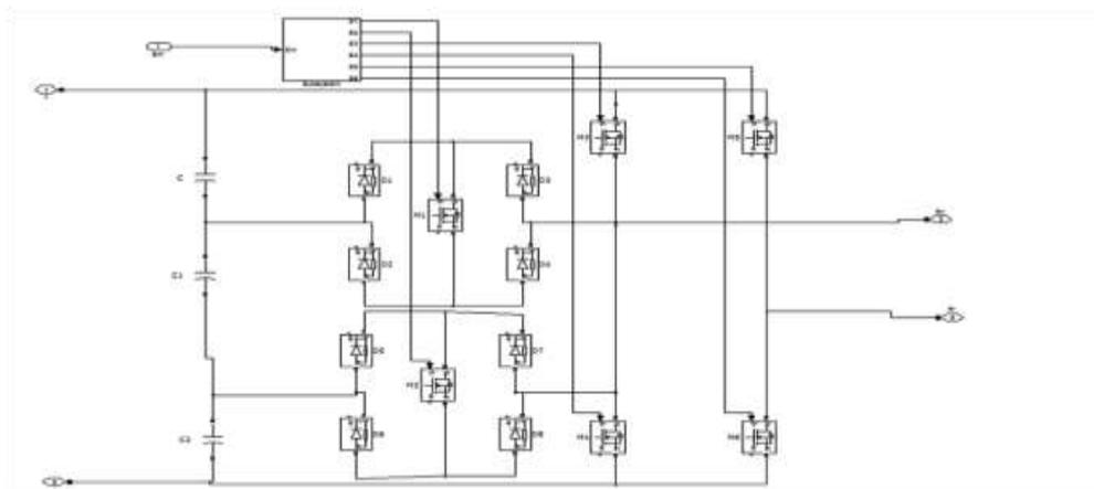
**Fig.14 Simulation Diagram of Modified Nine Level Inverter (MNL) Unit**
