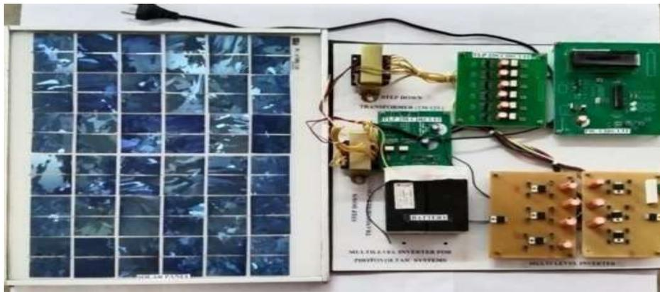
**Fig.19 Prototype model of PV based 9 level inverter**
