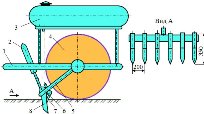
**Rice. 2. Hydromechanical sealing device**
