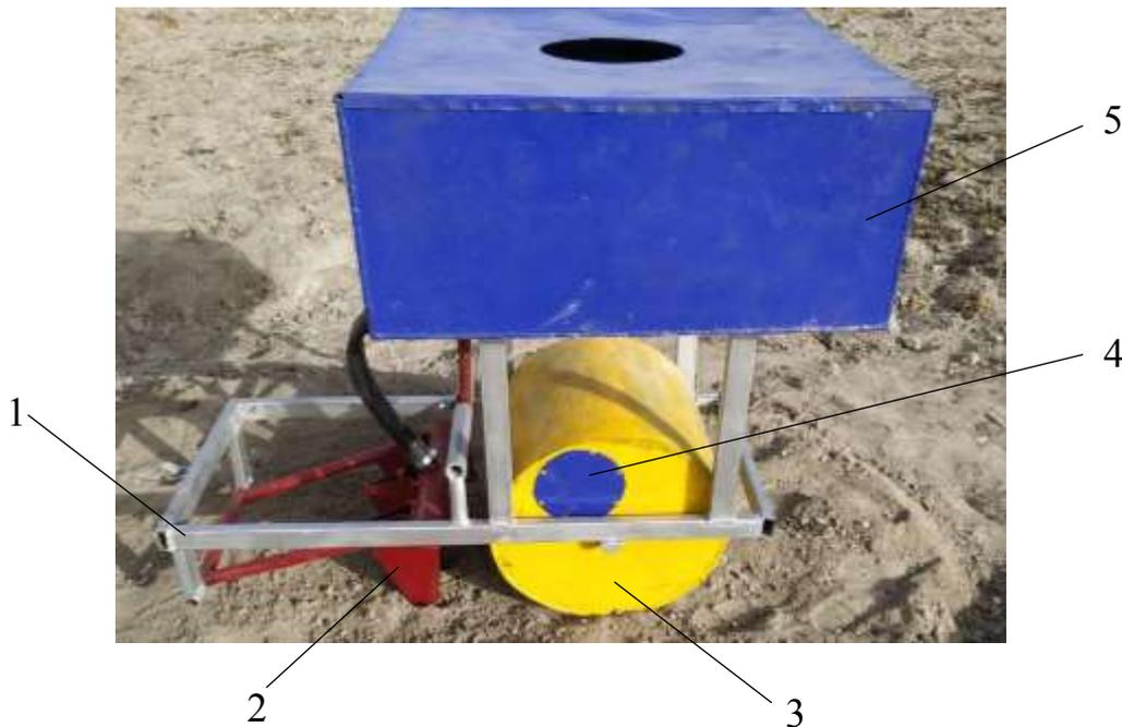
**Fig.5. General view of the soil-compacting body: 1-frame; 2-moisturizing body; 3-skating rink; 4-lid; 5-capacity for water.**
